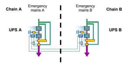
If A and B emergency mains are present and within tolerances, UPS A is synchronised on the emergency mains A and UPS B is synchronised on emergency mains B.
